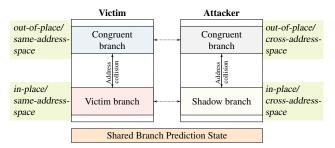
Figure 3: A branch can be mistrained either by the victim process (same-address-space) or by an attacker-controlled process (cross-address-space). Mistraining can be achieved either using the vulnerable branch itself (in-place) or a branch at a congruent virtual address (out-of-place).
