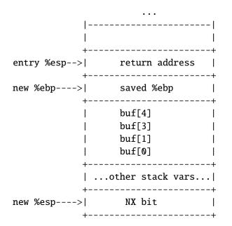
such that, as shown in the sample code above, an overflow attack in the frame will not overwrite the frame's NX bit.
