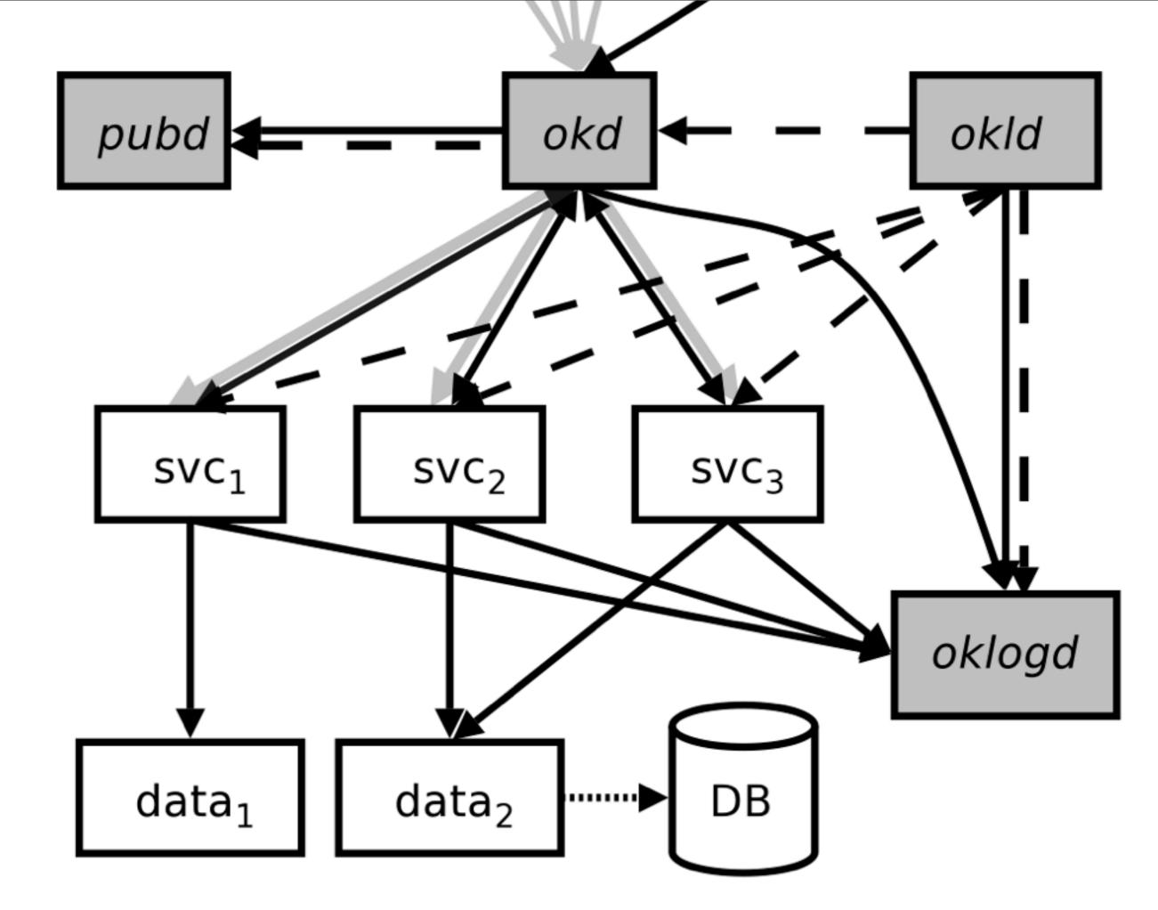
OKLD: Reads config file, opens 2 socket pairs (HTTP, RPC), forks, chroot, cd, setuid/gid/list, execs, sends server HTTP and RPC sockets to OKD.
