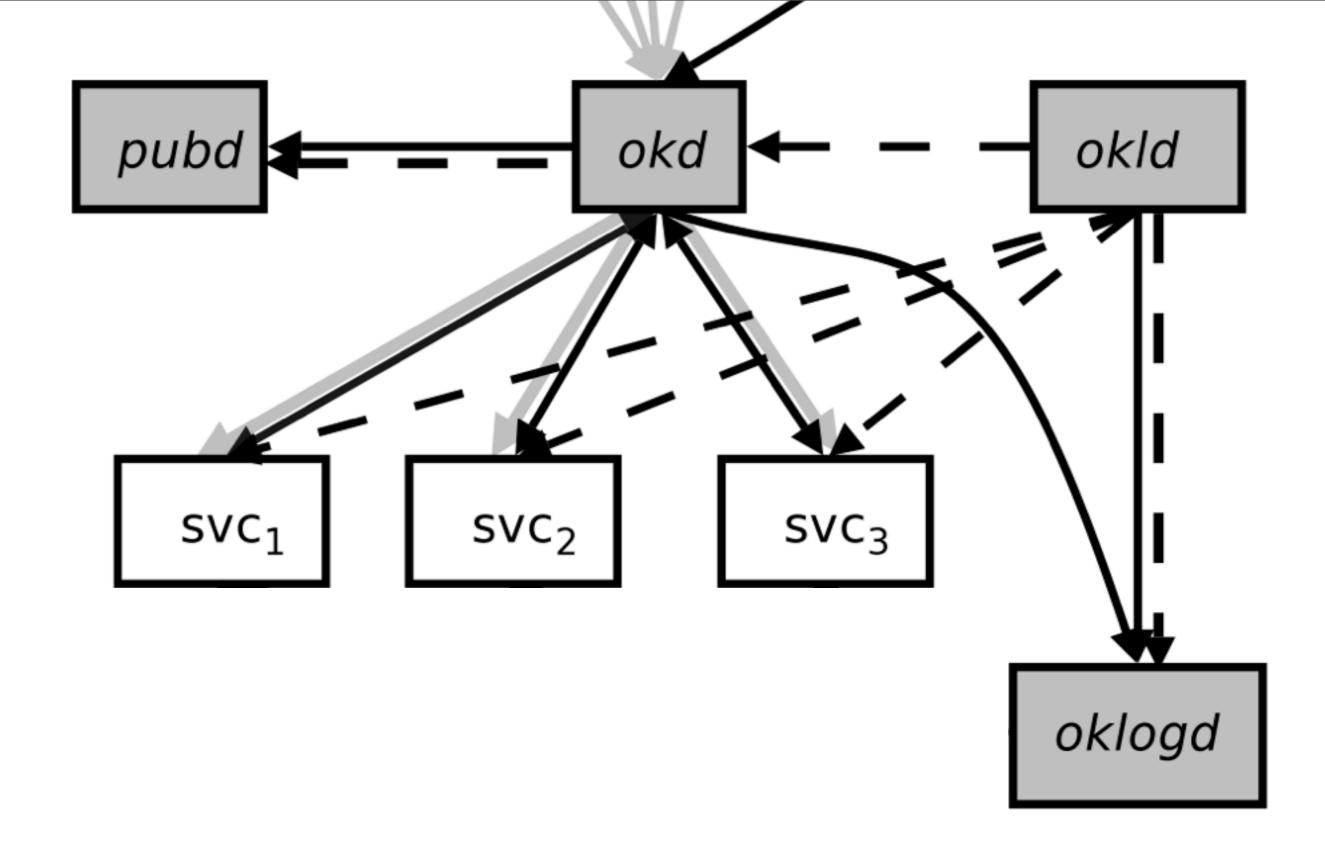
OKLD: Reads config file, opens 2 socket pairs (HTTP, RPC), forks, chroot, cd, setuid/gid/list, execs, sends server HTTP and RPC sockets to OKD.
