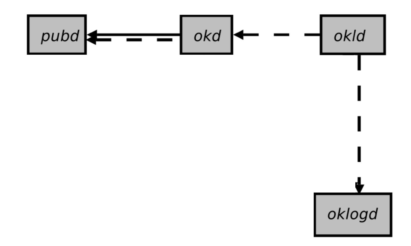
OKLD: Reads config file, opens 2 socket pairs (HTTP, RPC), forks, chroot, cd, setuid/gid/list, execs, sends server HTTP and RPC sockets to OKD.
