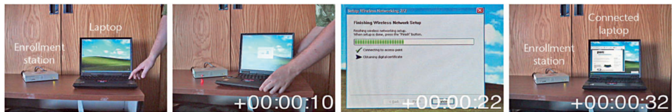
Figure 2. Gesture-directed automatic configuration. The user briefly aligns a laptop's infrared ports and an enrollment station to start a fully automated setup.
