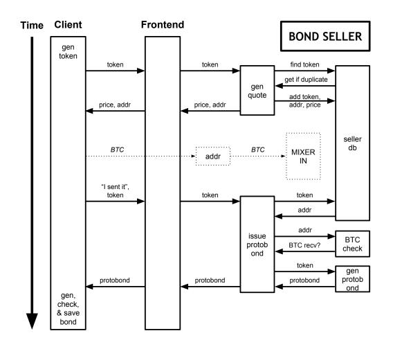
Figure 2: The seller privilege separation. Each box is a separate process running under a distinct UID.
