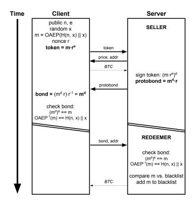
Figure 1: The entirety of the Dryer21 protocol in a nutshell.
