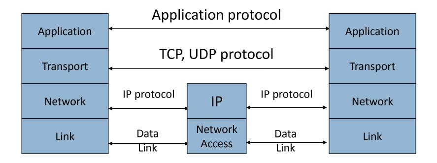
Transport layer provides *ports*, logical channels identified by number
