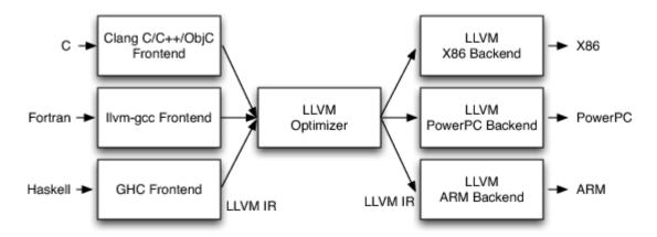
The frontend will consume a higher level language and produce a specialized intermediate representation (IR), denoted as LLVM IR. This IR can then be acted on by optimization routines. Finally, the IR is passed to a backend where it is transformed in to native instruction code for a target platform. Of note, the IR is inherently platform agnostic. Our transformations happen in the middle, as an 'optimization'.
