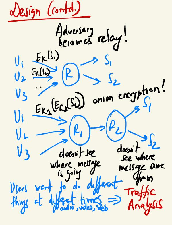
Traffic (orrelation Signal V, GT  $\frac{1}{2}$ observing both sender & recipient shows correlations in traffic volume, traffic timing, and causality S- sent same volume cont- at the same fime puter, foibas. OR in broduce random delaifs? OR dummy messages?
