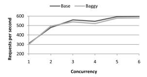
Figure 16: Throughput of NullHTTPD web server for varying numbers of concurrent requests.
