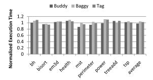
Figure 19: Normalized execution time on AMD64 with Olden benchmarks.
