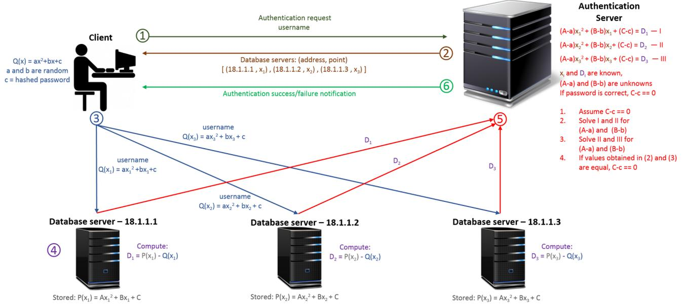
**Figure 3:** The authentication protocol in our distributed password storage system for  $k = 3$ .
